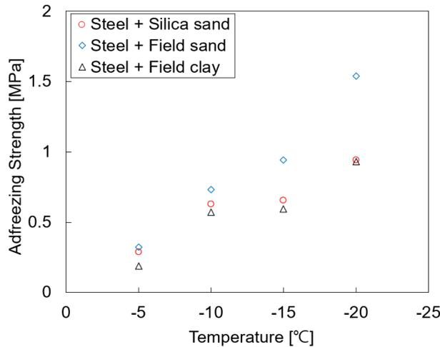
Fig. 3 Relationship between adfreezing strength and temperatures with steel ring structure at 16% and 3 of water contents
