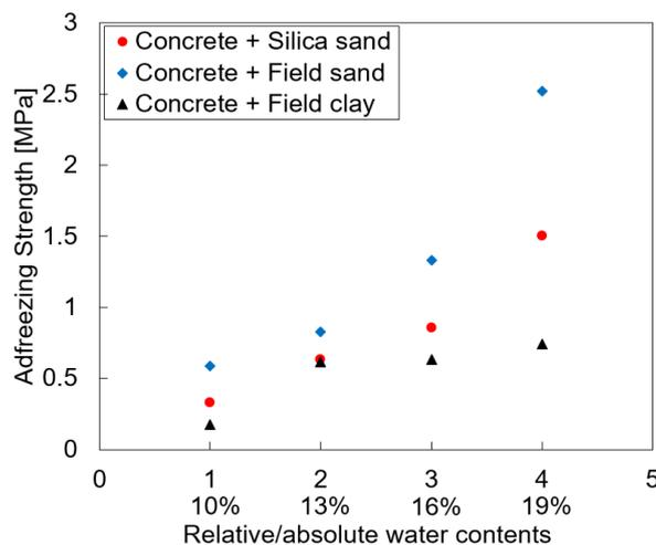
Fig. 2 Relationship between adfreezing strength and water contents with concrete ring structure at  $-15\text{ }^{\circ}\text{C}$
