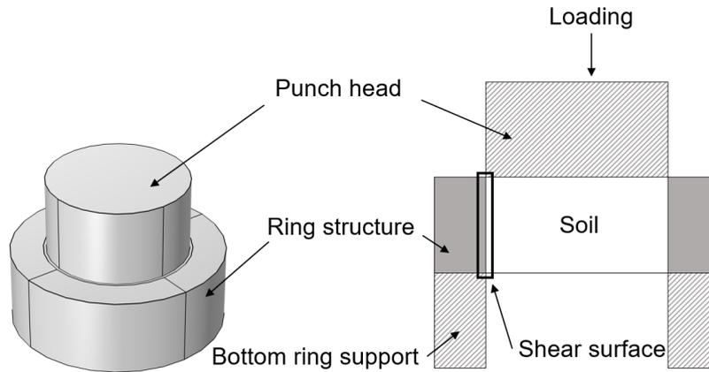
Fig. 1 Schematics of punch shear test setup and shear surface
